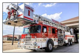
Many ladder trucks combine the operational capabilities of a ladder truck and the waterpumping ability of a fire engine and provide five main firefighting functions: pump, water tank, fire hose, aerial device and multiple ground ladders.
